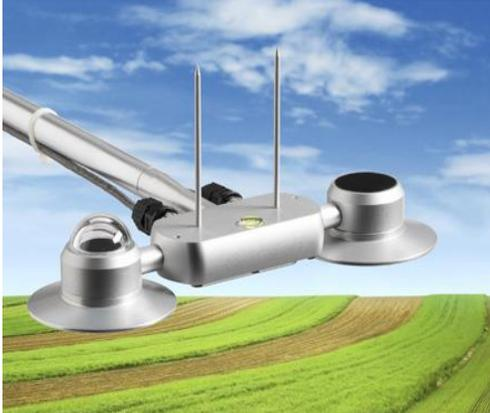
LP NET 14 is a 4-component Net-Radiometer for the measurement of the net radiation between  $0.3\mu\text{m}$  and  $45\mu\text{m}$ . The net-radiometer consists of two pyranometers (one for the measurement of the global radiation and the other one for the measurement of the reflected solar radiation) and a pair of pyrgeometers (one for the measurement of the infrared radiation emitted by the sky and the other one for the infrared emitted by the ground surface).
